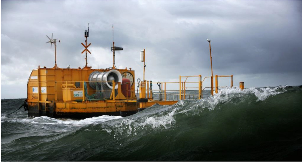
Fig. 18. 1:4th-scale prototype of BBDB (the OE Buoy) equipped with a Wells turbine being tested in Galway Bay, Ireland, about 2008.
