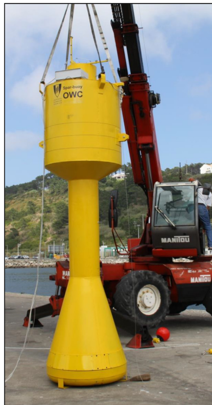
Fig. 21. Spar-buoy OWC. Cross section and 1:16th-scale model tested at NAREC, UK, in 2012.
