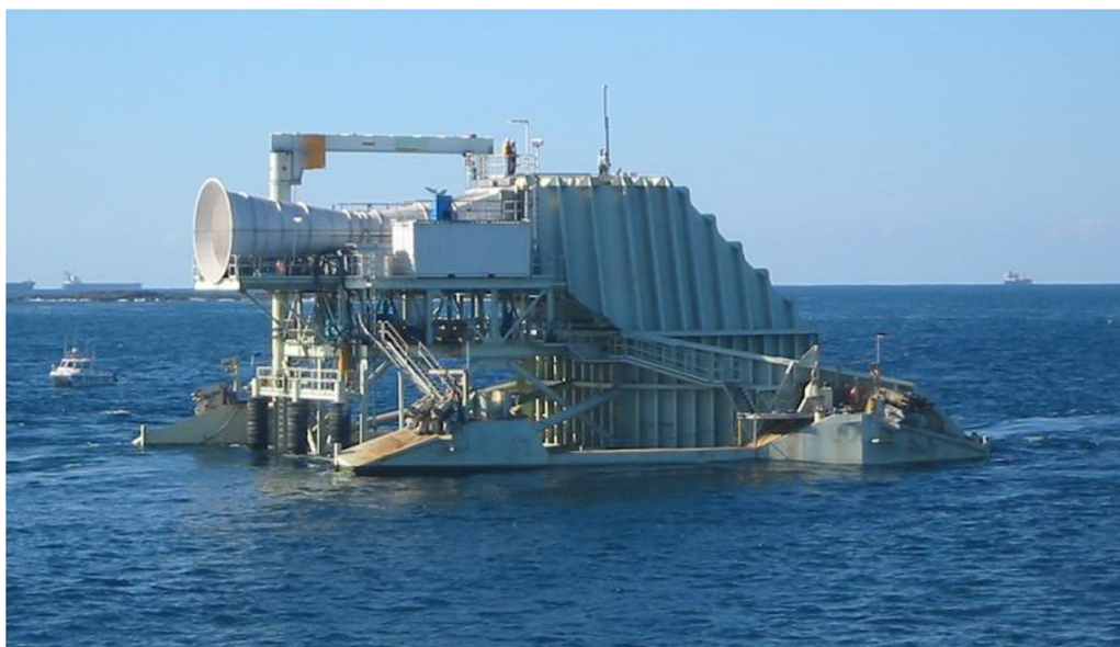
Fig. 15. Oceanlinx bottom-standing OWC, Australia, about 2005.
