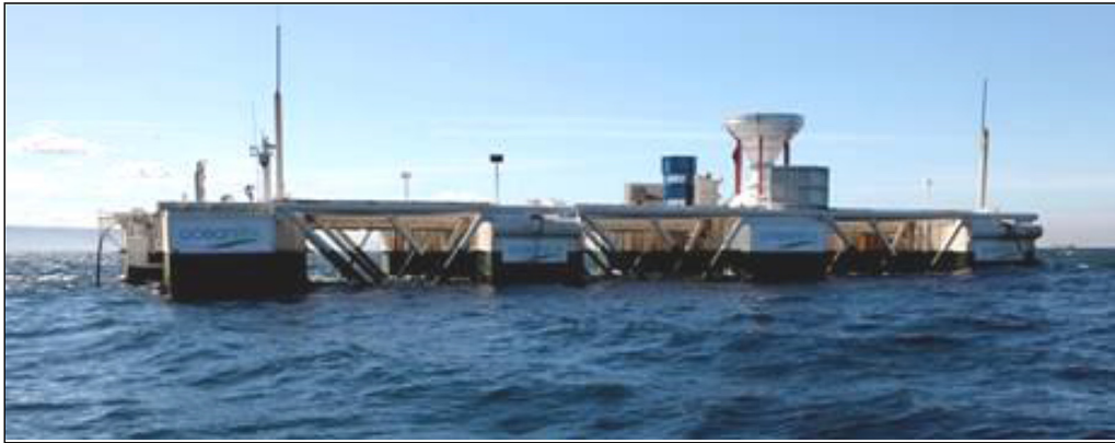
Fig. 20. 1:3rd-scale Oceanlinx Mk3 multi-chamber floating OWC device, 2010.
