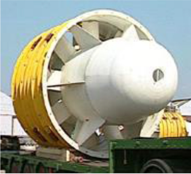
Fig. 40. 2 × 500 kW contra-rotating Wells turbine of OSPREY, about 1995.
