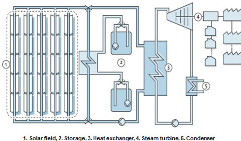
Fig. 1. Schematic illustration of Andasol 3.
