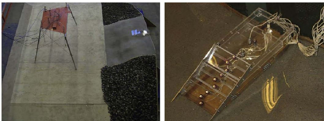
Fig. 7. Physical setup of 3D laboratory tests on wave loadings. On the right the model in scale 1:60 equipped with pressure transducers.
