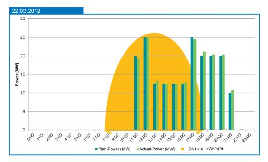
Fig. 4. Dispatchability test on 22 March 2012
