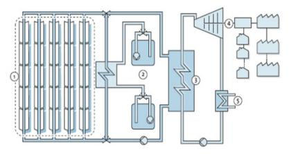
1. Solar field, 2. Storage, 3. Heat exchanger, 4. Steam turbine, 5. Condenser
