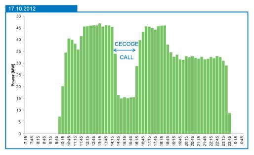
Fig. 6. Power gross output of Andasol 3 during power reduction request.
