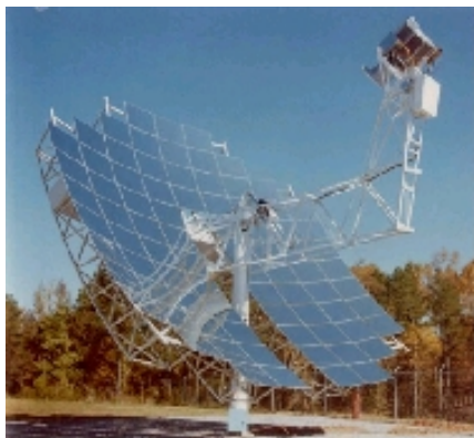
The McDonnell-Douglas dish/Stirling system
