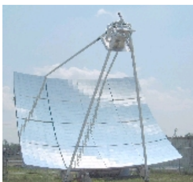
HiTek's 14 m 2 dish prototype
