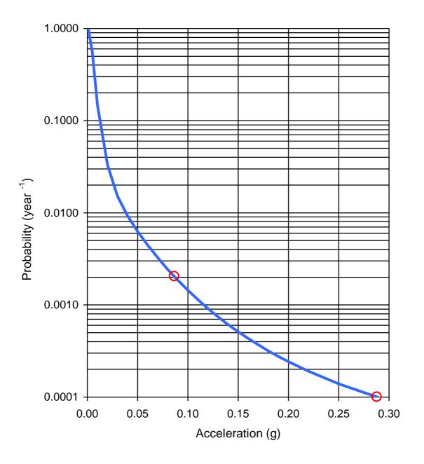
Figure 2–2 Spectral acceleration, T = 0 s
